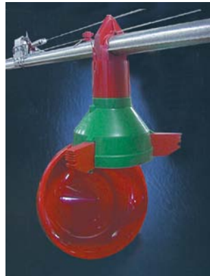
Single handle adjusts cones on 300 feet (92 meters) of feeder line.
